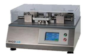
The device measures the number of folds until the sample breaks. The test requires two samples to be tested simultaneously. It is equipped with a touch screen displaying the temperature, the number of folds and statistical values. The heads are equipped with temperature sensors to convey the temperature inside the heads.
