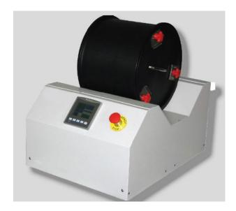
The Hexapod TumblerTester is a popular apparatus used internationally for the evaluation of the appearance retention of carpets. The unit provides a rapid and convenient method of test to recognised standards and carpet samples can be tested with or without underlay. The new generation model includes a colour touch-screen making the operation even easier.
