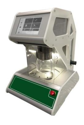
The Bursting Strength Tester is a pneumatic instrument, it measures the required pressure necessary to burst specimens and distension prior to bursting. The sample distension height is measured by means of laser technology. All burst tests performed with the instrument conform to the main international standards; these are preset or freely programmable to suit individual/custom made settings.
