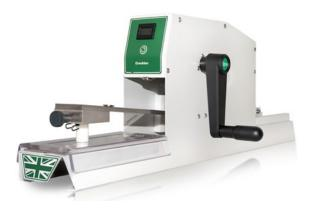
The conventional design of the *CROCKMETER* has been enhanced using advanced materials to minimise friction at the crank pin and arm guide whilst eliminating the requirement for lubrication and the potential for contamination. The *CROCKMETER* is constructed from materials that are extremely durable to ensure a long service life.
