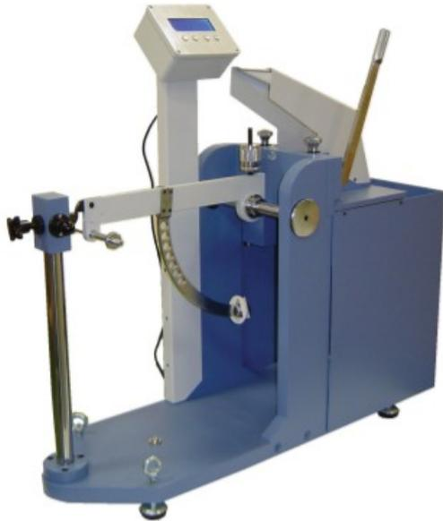
For measuring the required energy to puncture corrugated board and cardboard.
