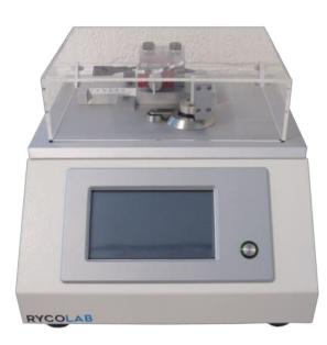
For the determination of bending resistance and stiffness of paper and paperboard
