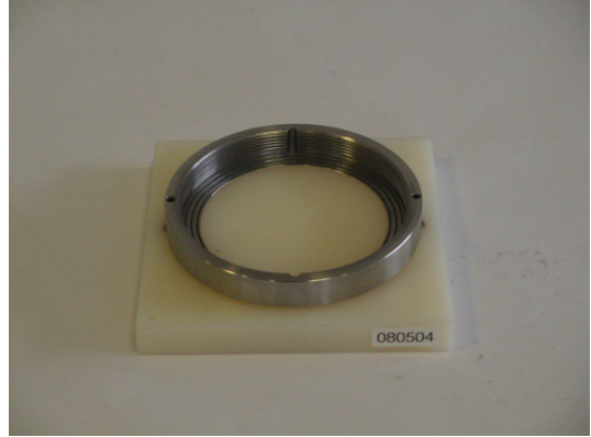
Step 2: Lay outer clamping ring onto the base plate.
