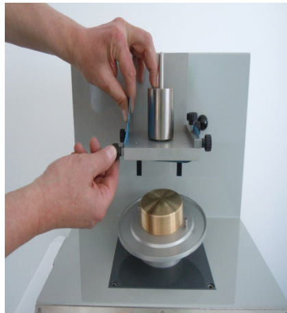
Step 3: Sandpaper with set screws tighten on both sides.
