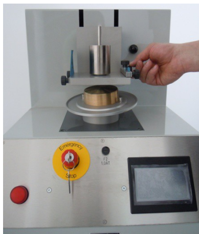
Step 5: The jig with the clamped sandpaper carefully on the taper.
