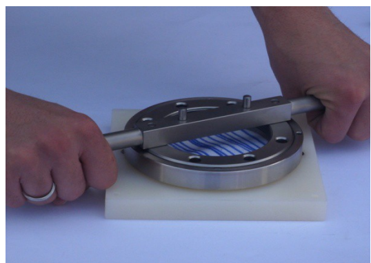
Step 6: Tighten up the clamping ring with the clamping spanner.
