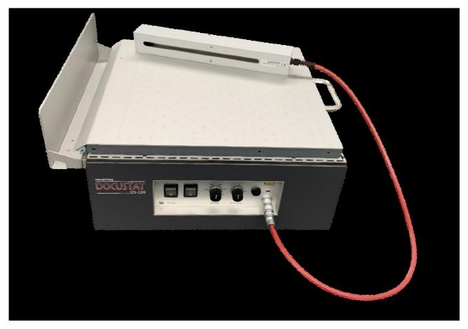
Due to the rather large dimensions of the examination unit (450x440 mm), the Docustat DS-220 system can be used for small and large examination objects. The supplied plastic film, type IW, allows the system to be used for a variety of applications such as: Securing writing impression marks (grooves) on paper-like surfaces.
