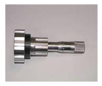
During the test, a ball is manually pressed into the test specimen. The stretching is continued until the scar bursts. When testing the heat heat resistance of patent leathers, the test specimen is first stretched. Then is then heated and examined for any bursting of the coating layer.
