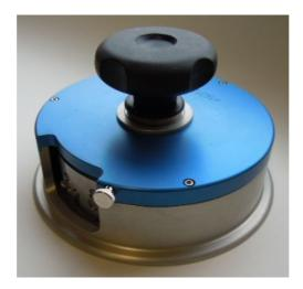
Only a test specimen with a precisely maintained area dimension guarantees the reliable weight determination. That is why SCHRÖDER builds PS specimen cutters for you. Sharp, circularly guided knives produce true-to-size round specimens with absolutely smooth absolutely smooth edges. Even "critical" materials such as thin foils, tissue paper, corrugated cardboard, hosiery, nonwovens, carpets, artificial leather, fluffy or velvety fabrics can be cut without any problems.
